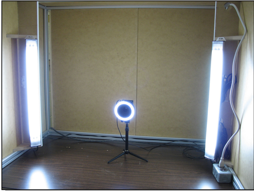
Figure 5.3: Interior lighting in the test cell consists of two 2 foot long, high frequency fluorescent lights, and one LED ring light mounted to the camera.
