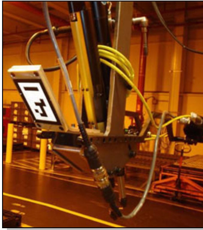
Figure 2.1: Semi-automated inspection systems assist a human operator by tracking tools to ensure they have completed all tasks at a particular assembly station (Wilson, 2006).
