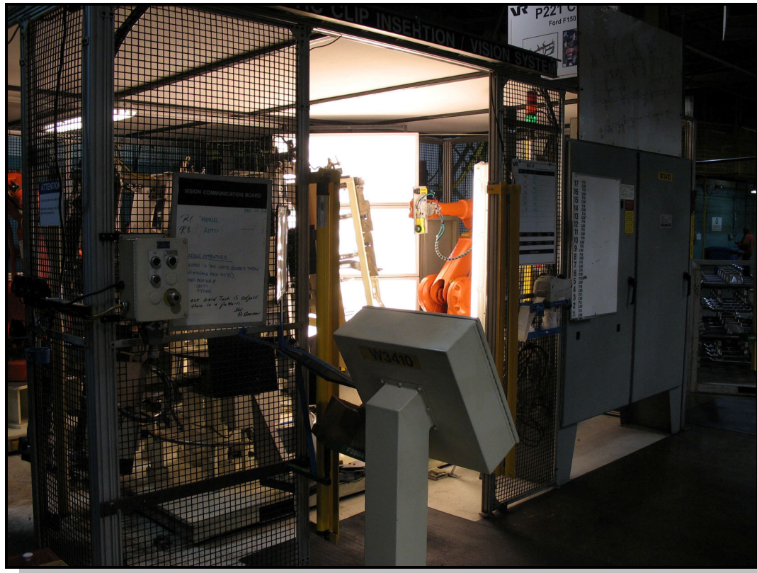
Figure 2.3: An example of an Automated Visual Inspection system installed at Van Rob Stampings. The system uses two cameras mounted on a robot (visible inside the cage) and displays the results to the operator via the console unit (foreground)
